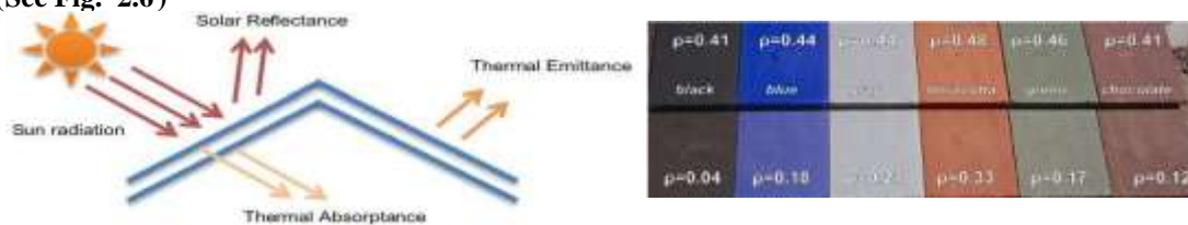
Figure 2.6. Showing Cool roof mechanism and Cool dark colour roofs
