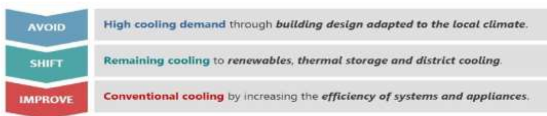
Figure 2.1. Steps for low carbon buildings
