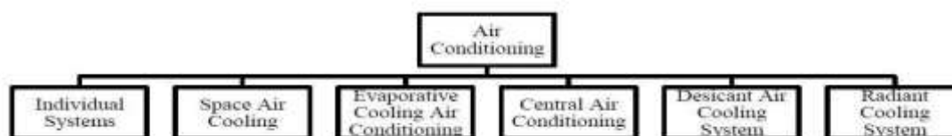
Figure 2.3. Categorization of air-conditioning systems
