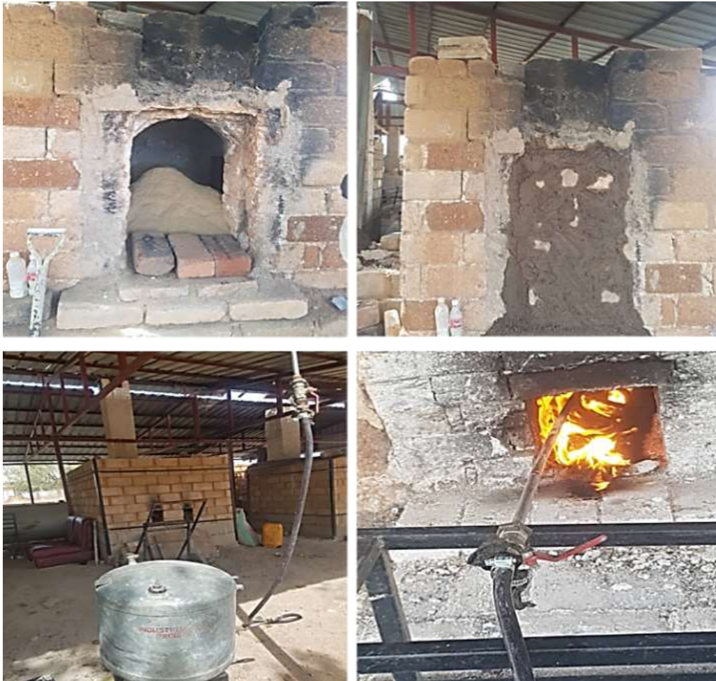
Figure 4: Local furnace for the production of rice husk ash
