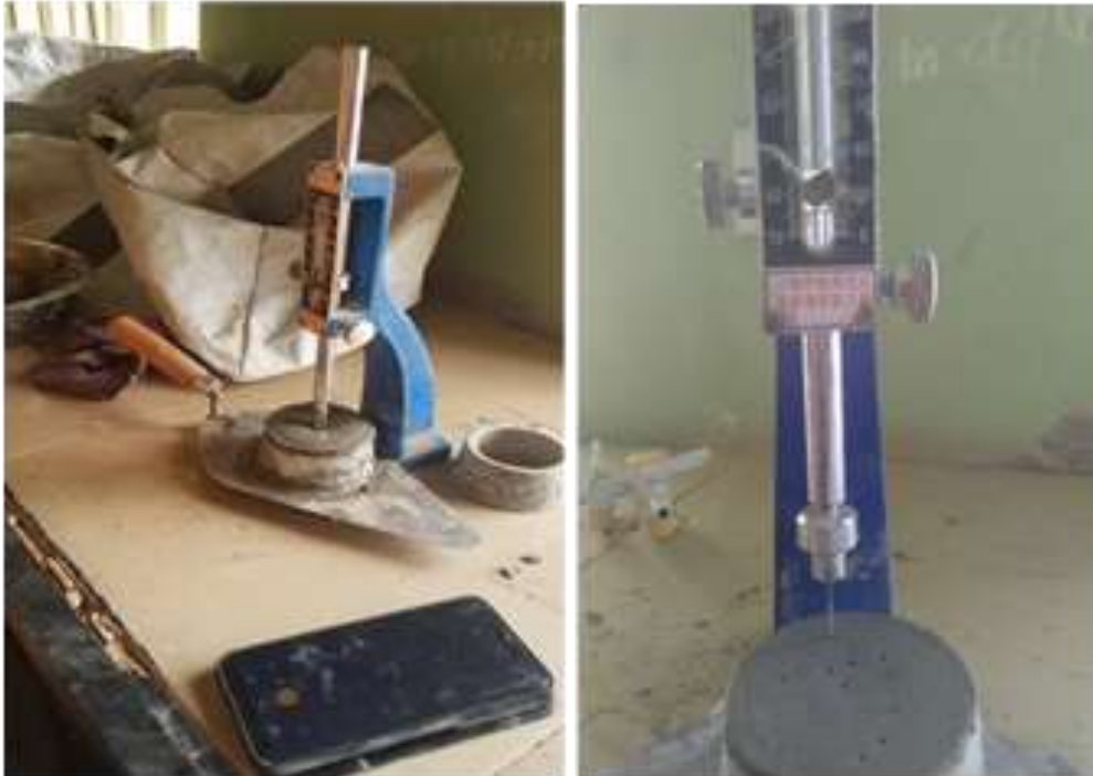
Figure 5: Testing of consistency and initial setting time
