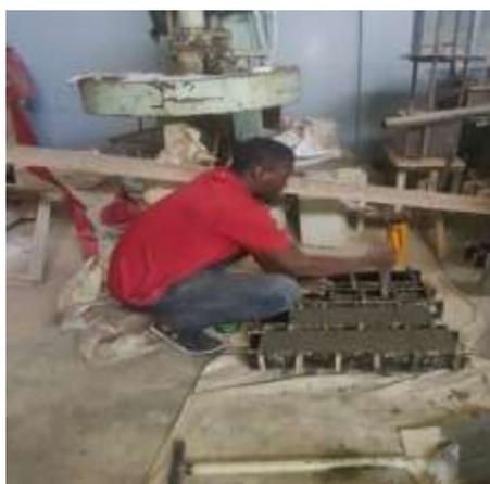
**Plate III:** Casting of the Cubes
