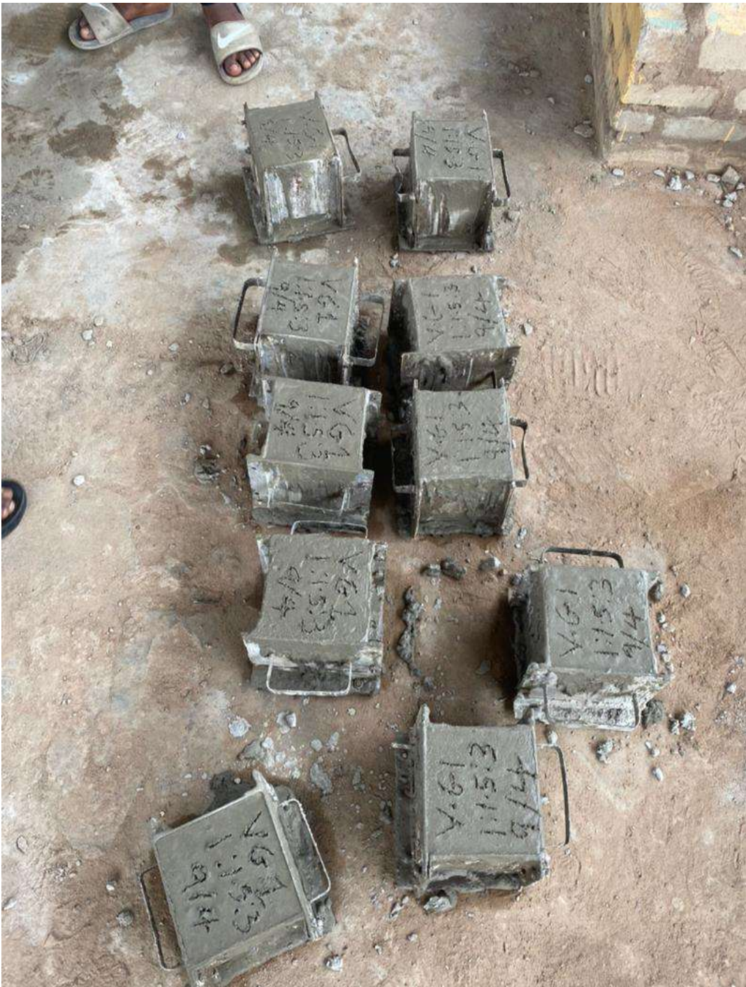
Plate 3 : Concrete cubes produced
