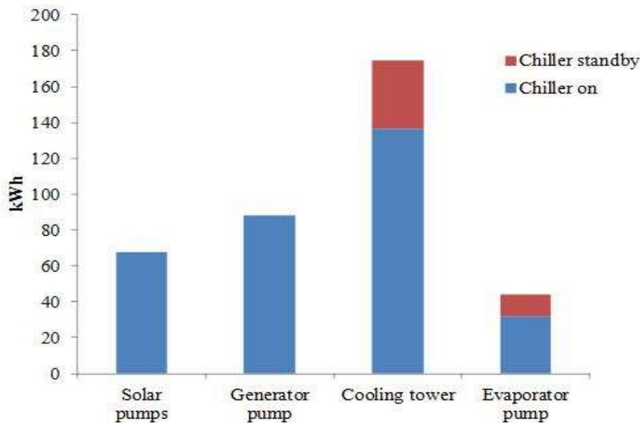
Fig. 2. Solar system electricity consumption (August 2011)
