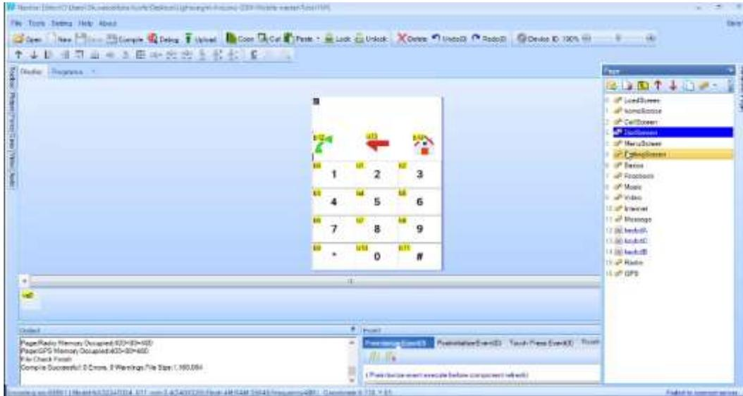
Fig. 2: Interface design using the Nextion Human Machine Interface (HMI)
