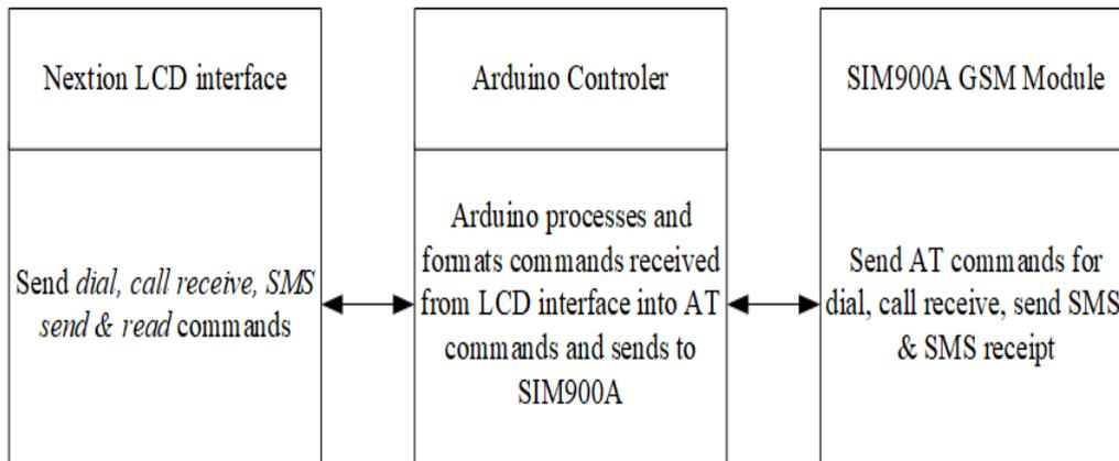
**Fig. 4 : Block diagram of operation of input/output interface, controller, and the SIM900A GSM module**
