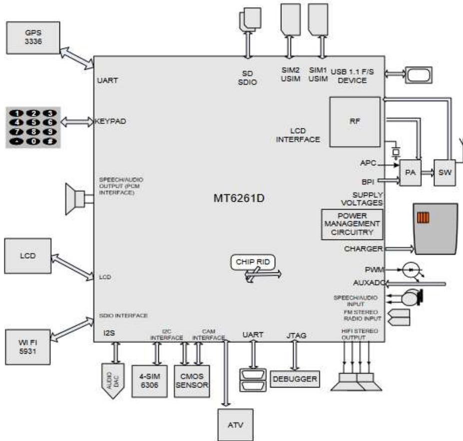
Fig. 1 - The MT6162 SoC Architecture (Dai, 2014)
