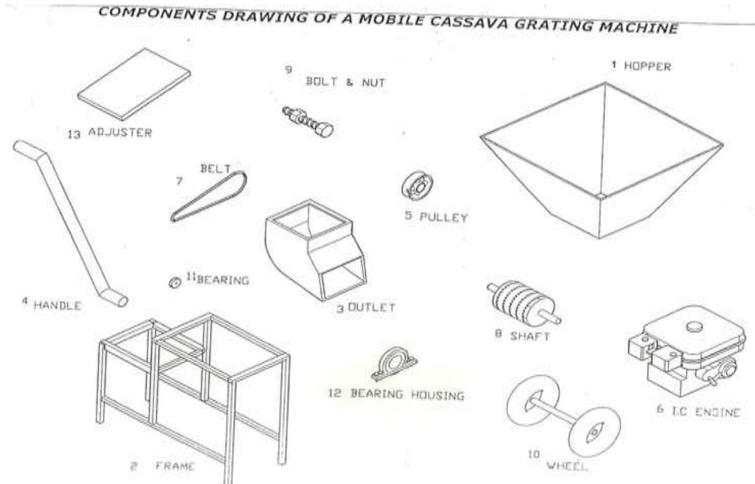
Figure 5. Components drawing of a mobile cassava grating machine. Source: (Aideloje, et. al., 2018)
