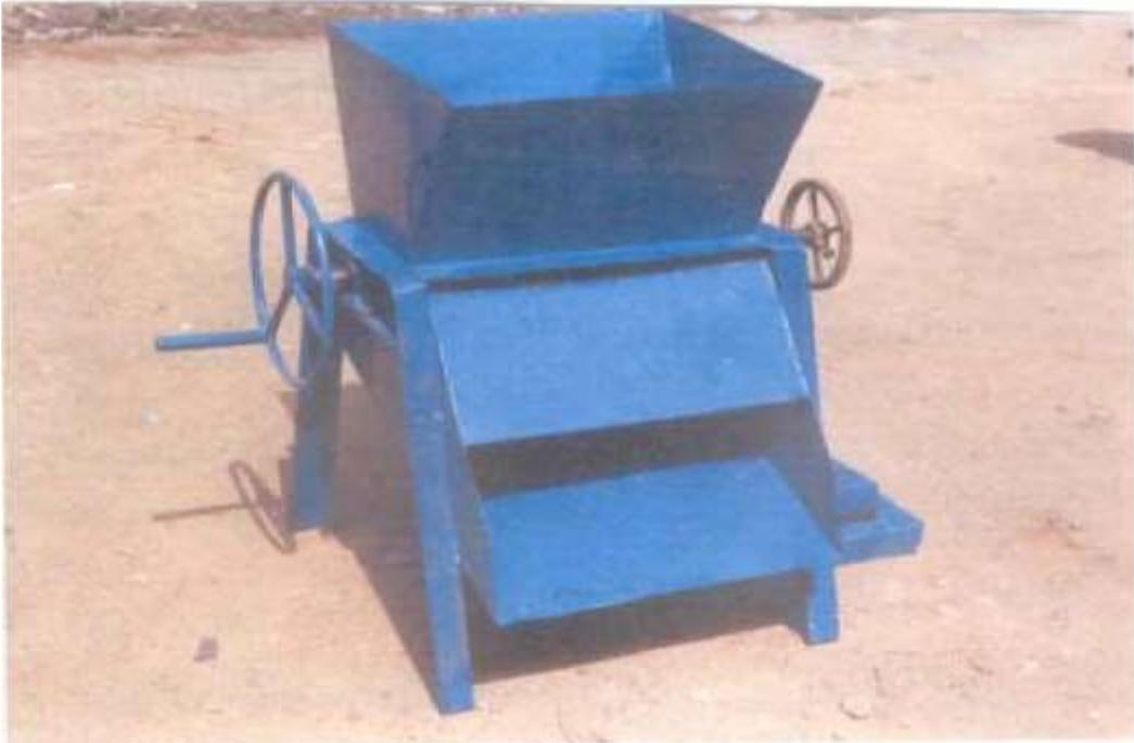
Plate 5. A Dual - Operational Cassava Grating Machine, Source: (Ndaliman , 2006)
