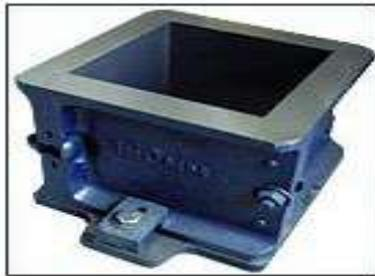
This concrete is poured in the mould and tempered properly so as not to have any voids. After 24 hours these moulds are removed and test specimens are put in water for curing. The top surface of this specimen should be made even and smooth. This is done by putting cement paste and spreading smoothly on whole area of specimen.
