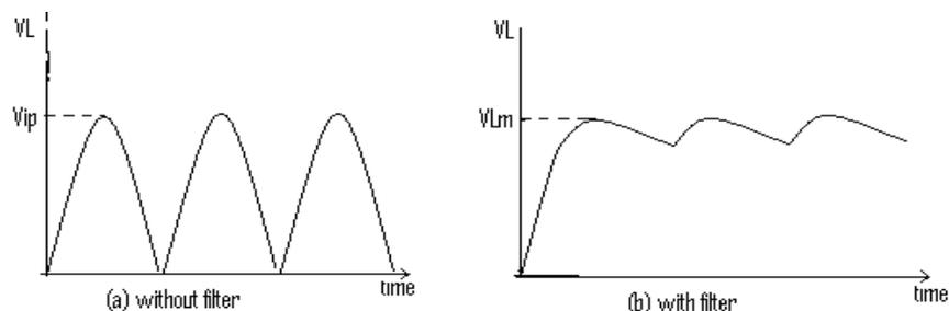
Figure 6: Filtering action of a capacitor filter. (Arbor, n.d.)
