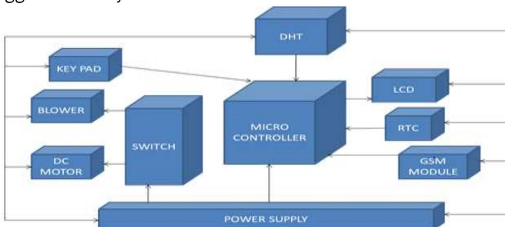
Figure 4: Block diagram of the hardware design
