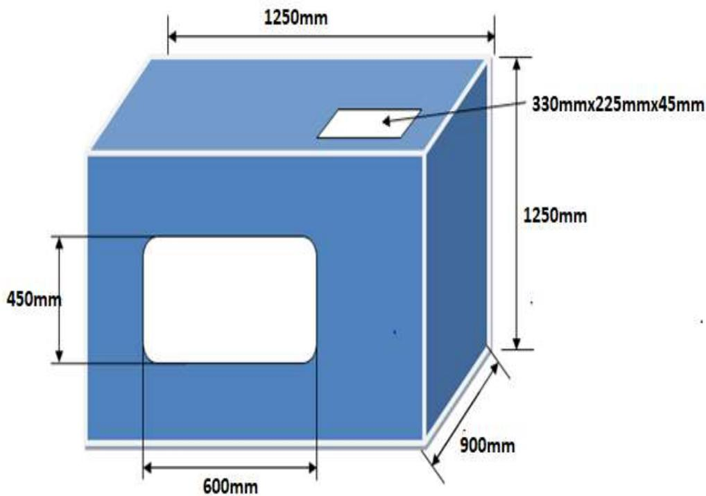
Figure 2: Casing of incubator
