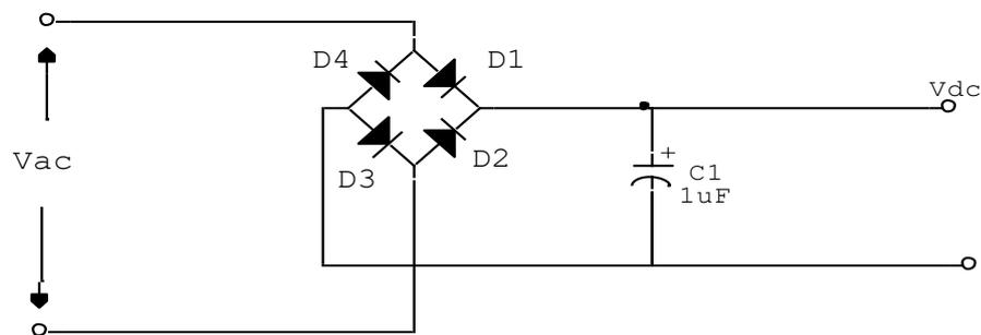
Figure 5: Full wave bridge rectifier. (Arbor, n.d.)
