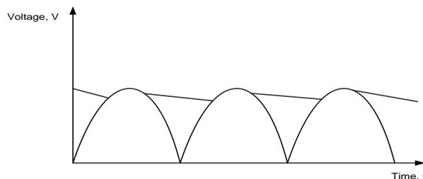
Figure 7: Rectified and Filtered Output. (Arbor, n.d.)
