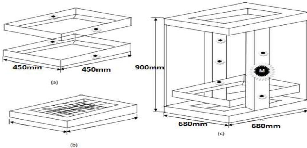
Figure 3: Shows the design of the (a) Egg Tray, (b) Egg Crate and (c) Egg Frame
