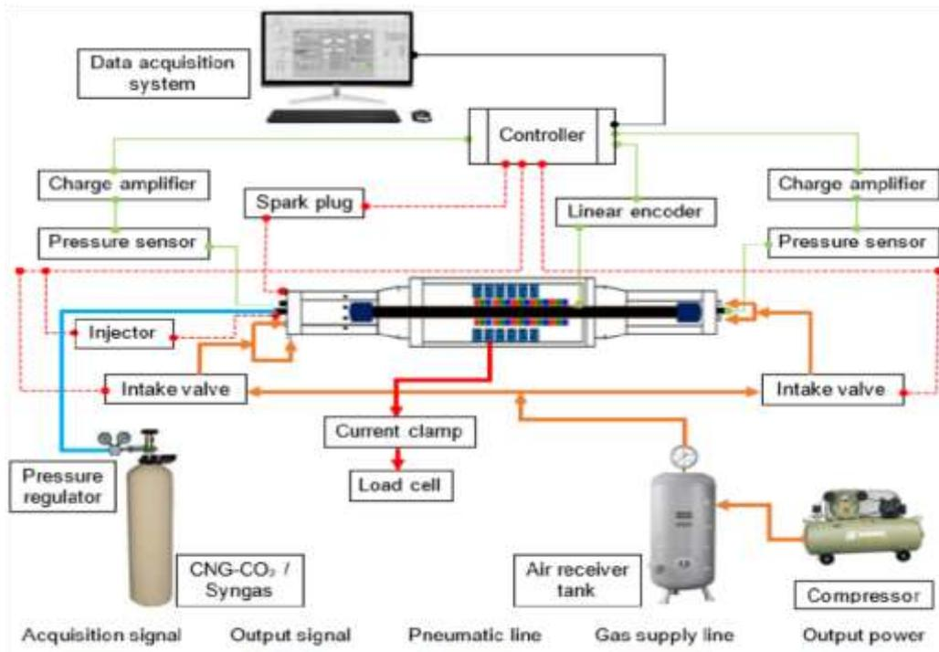
Fig. 1: The schematic of the experimental setup of the FPLG engine
