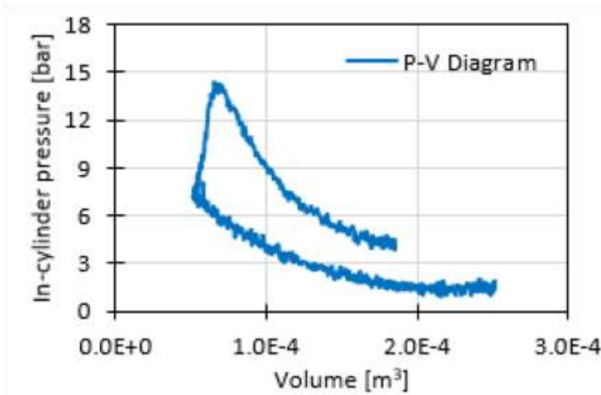
Fig. 5: Effect of syngas on FPLG performance: pressure-volume (p-v) diagram
