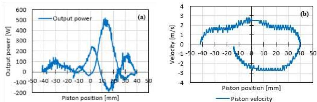
Fig. 4: Effect of syngas on FPLG performance: (a) output power and (b) piston velocity
