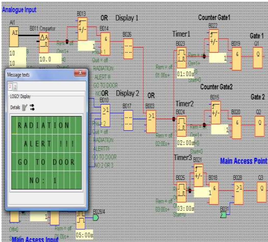
Fig 14: Analogue input test
