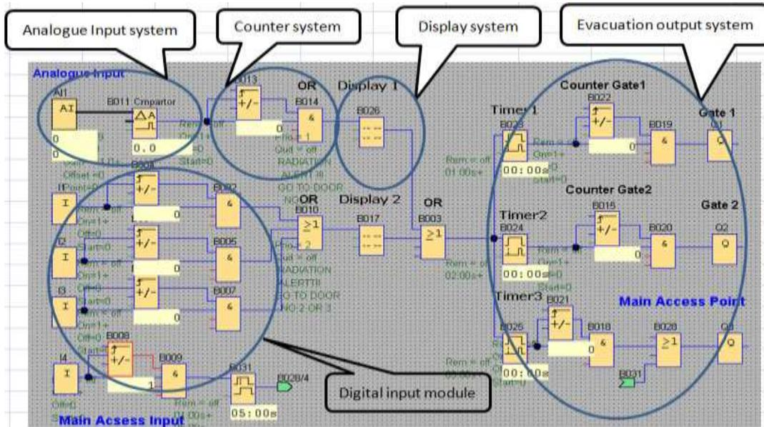
Fig 5: System Circuit Diagram (Modules of the design)
