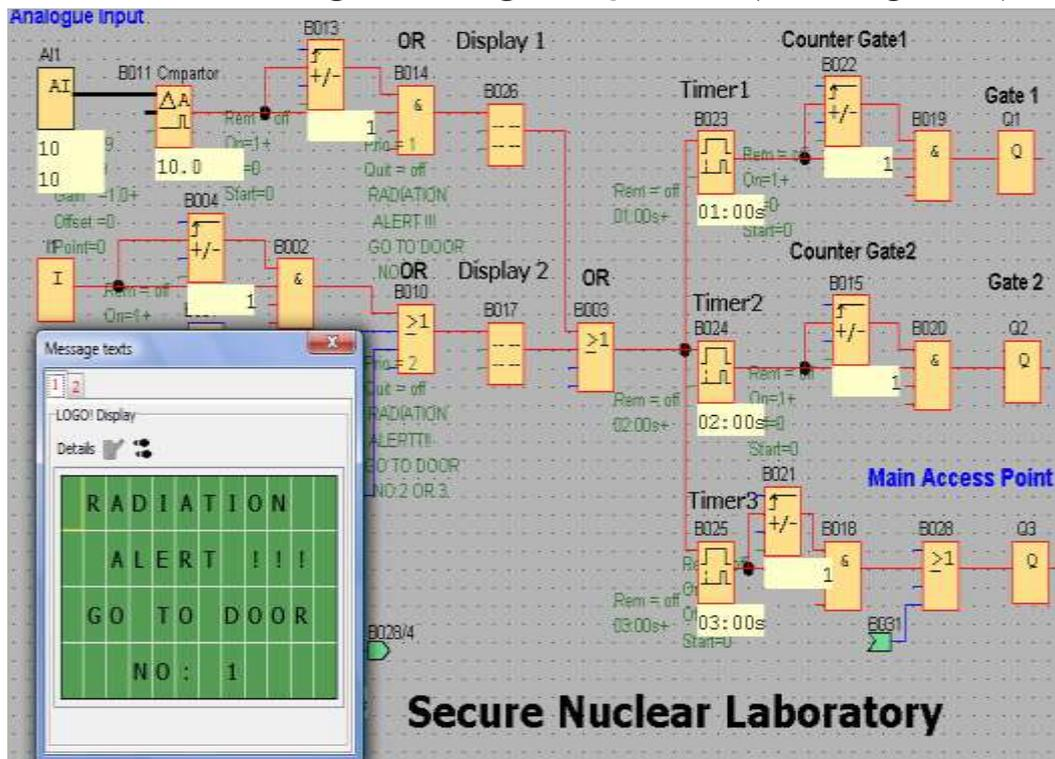
Fig 16: Simultaneous Analogue and Digital Input Test (With Logo Soft)
