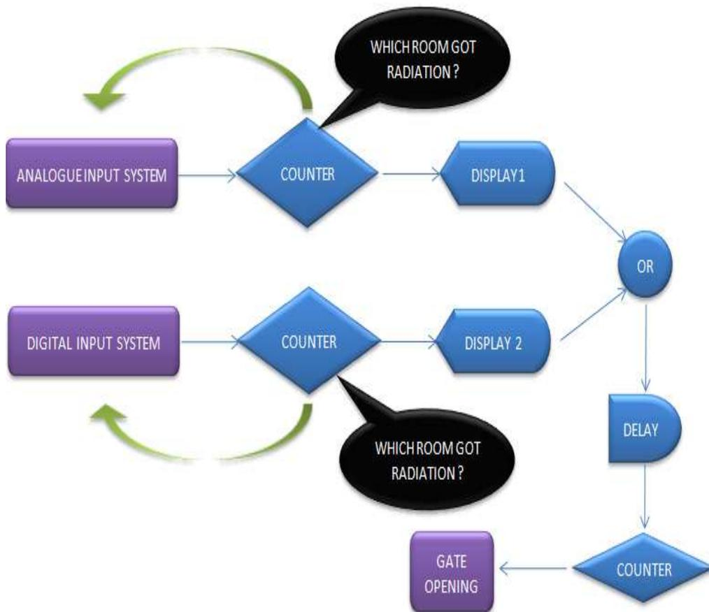
Fig 4: Flow chart for emergency evacuation system.
