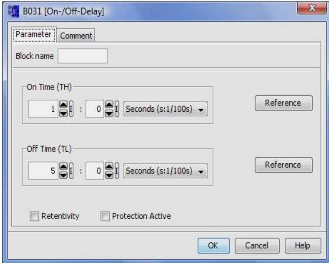
Fig 2: Access control timer (BO31) configuration
