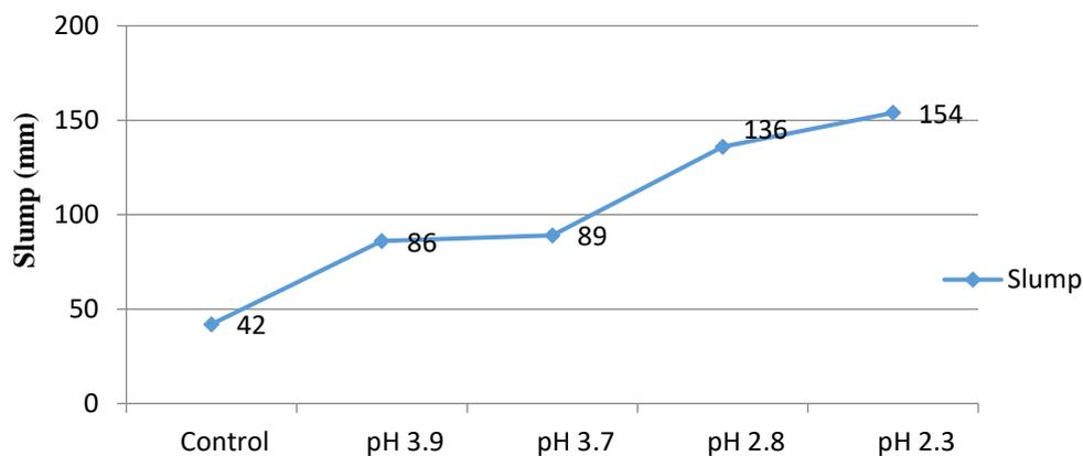
Figure 2: Slump heights versus pH values of locally made EM-A content
