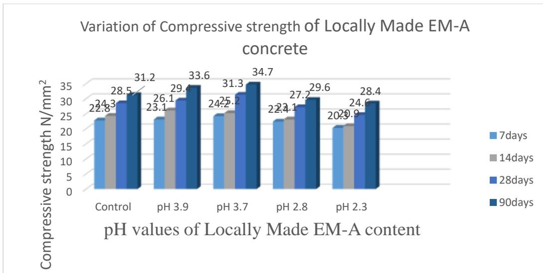
**Figure 3: Compressive strength versus locally made EM-A content at different pH values**
