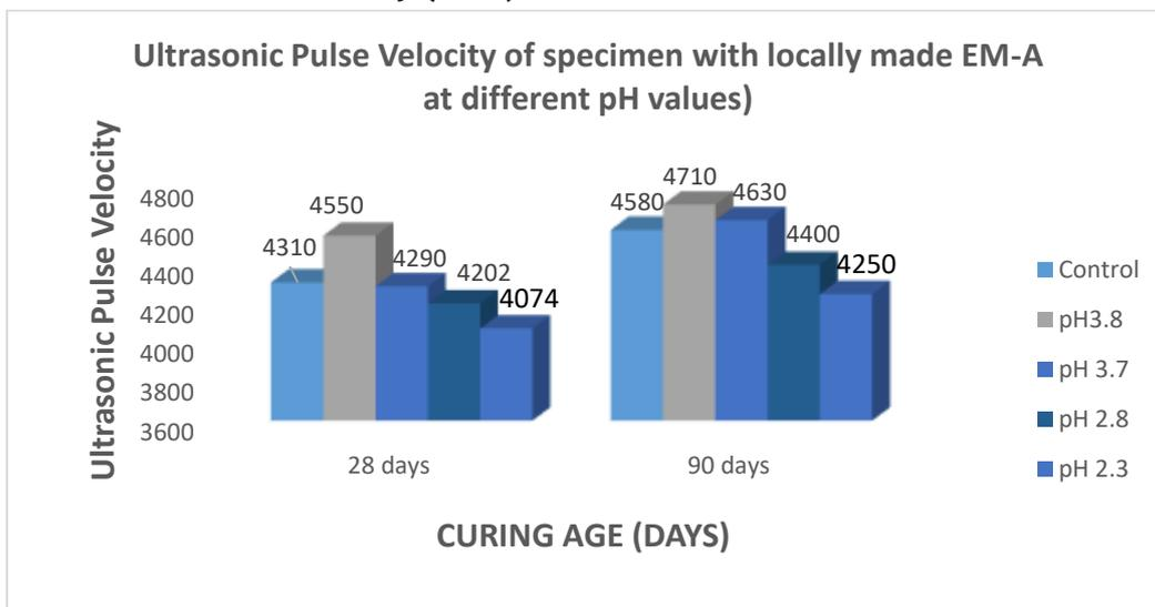
Figure4: Ultrasonic Pulse Velocity of specimen with locally made EM-A at different pH values
