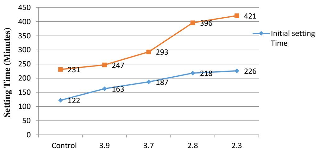
**Figure1:** setting time versus pH values of locally made EM-content
