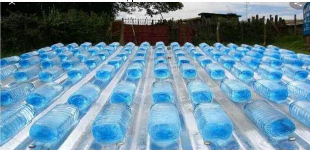
Plate 1: SODIS – Exposing water to sunlight in PET plastic Bottles
