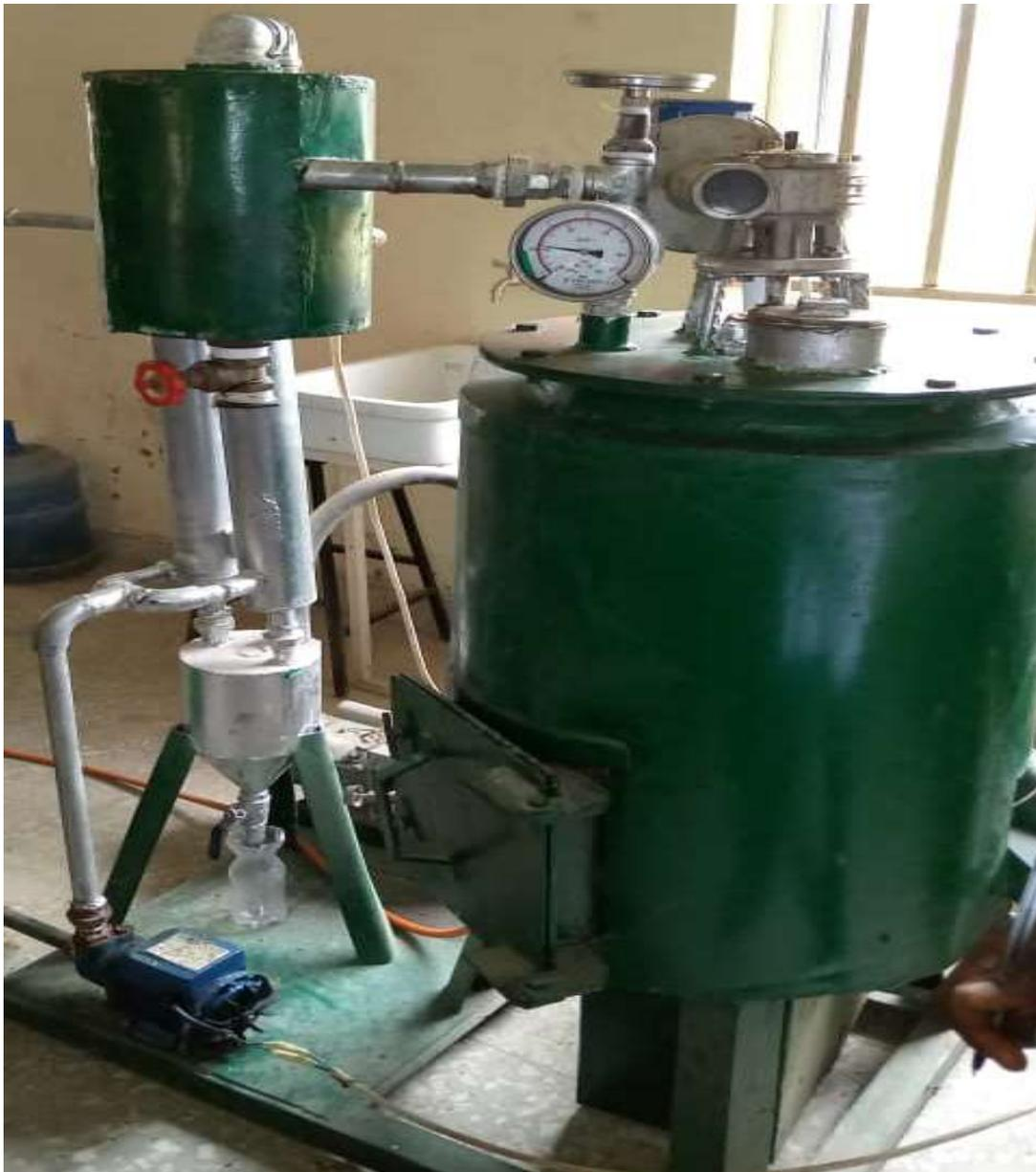
Fig 2: vacuum pyrolysis unit
