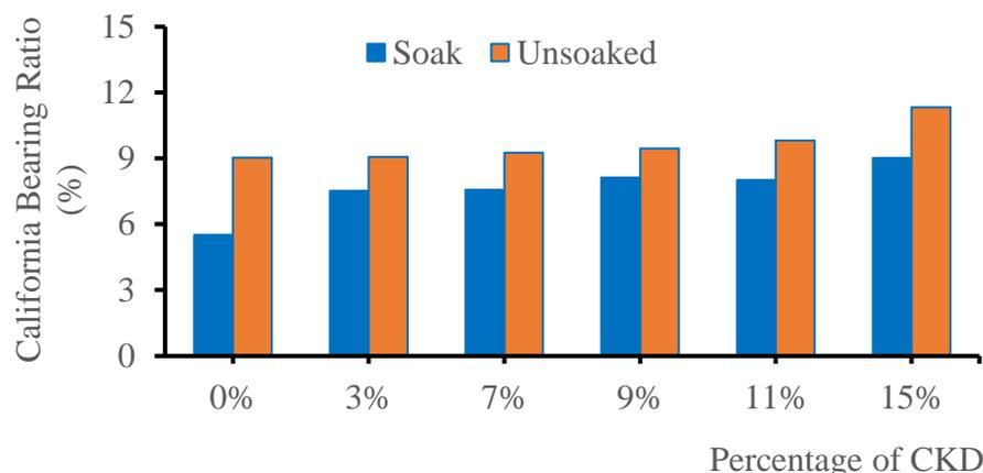
Fig. 3: Results of CBR Test
